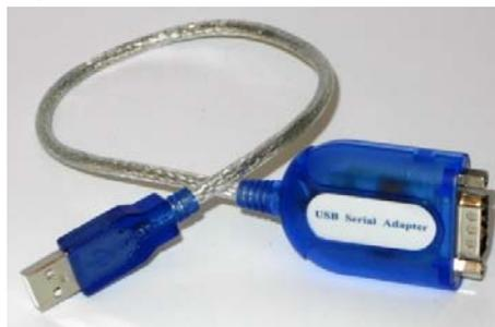
**Figure M-1** USB serial adapter
