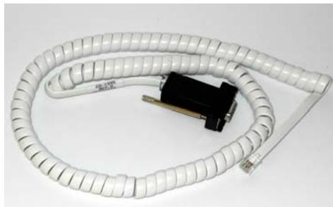
**Figure M-3** RJ-12 adapter and cable
