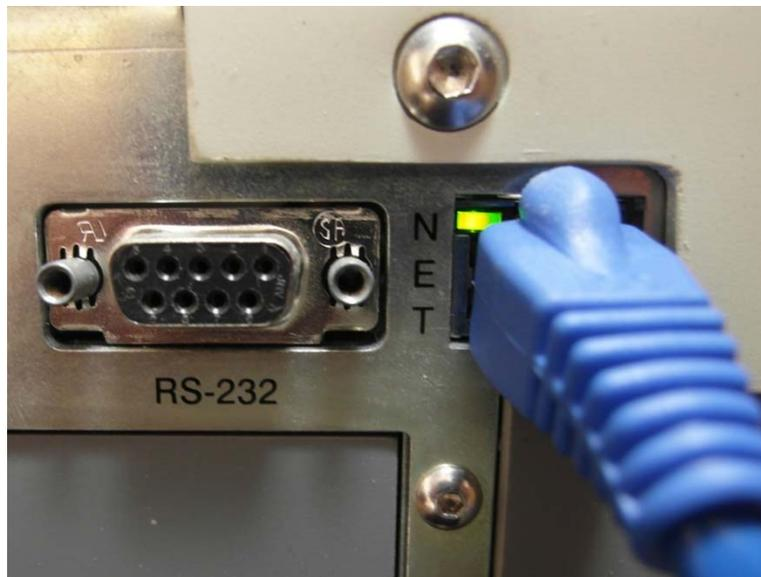
**Figure L-1** Ethernet port connectivity LED
